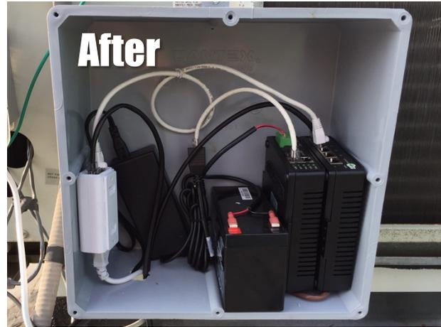
A Ubiquiti Rocket (top right) had been set up to communicate with just one Ubiquiti NanoBeam. This is overkill, to say the least. The Rocket has a 120-degree range; it's designed specifically for use with multiple NanoBeams.
